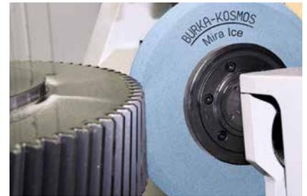
+ **Cool grinding:** The use of new grain qualities and the new high-strength bond system guarantees particularly cool grinding.
