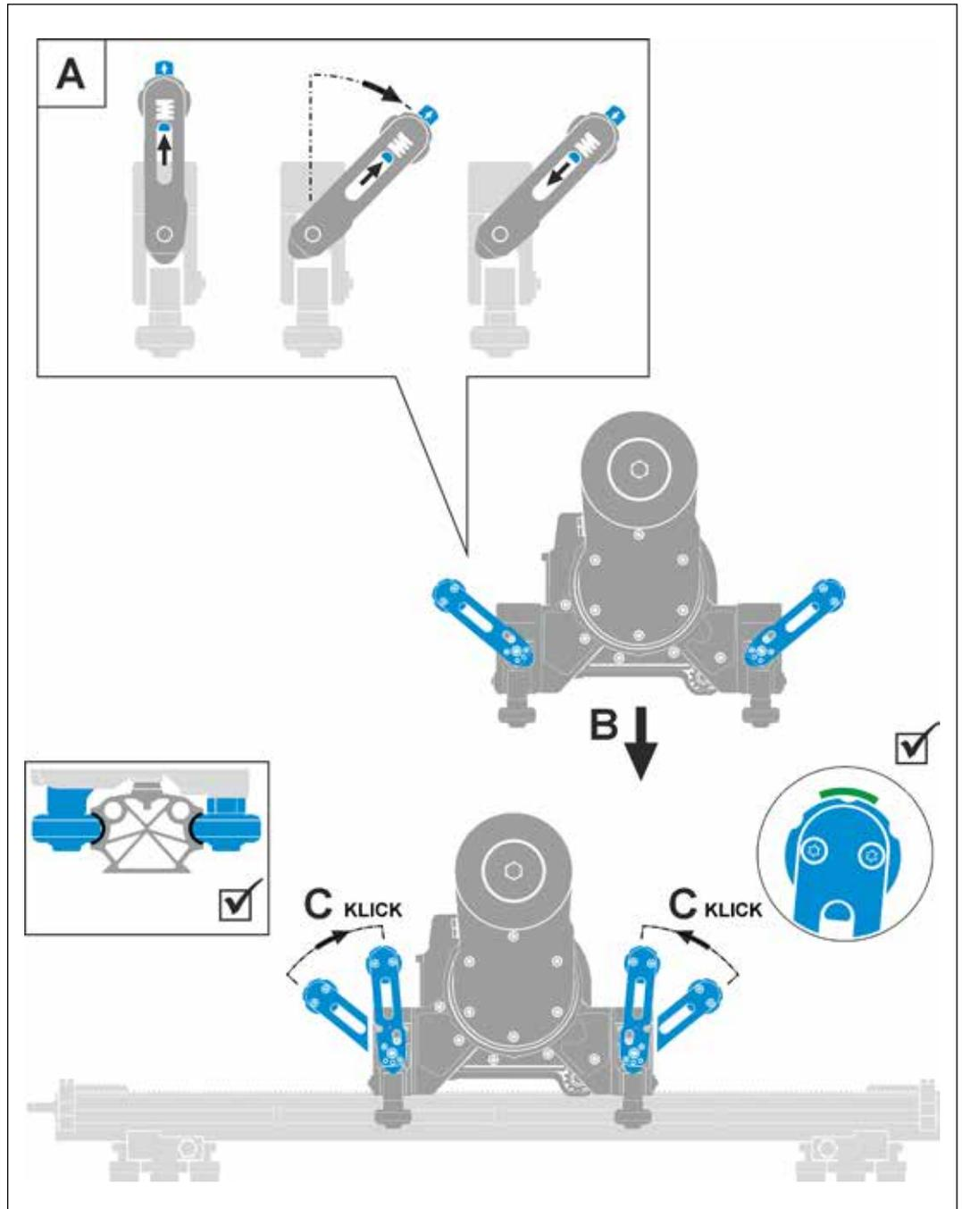
Mounting the wall saw head
