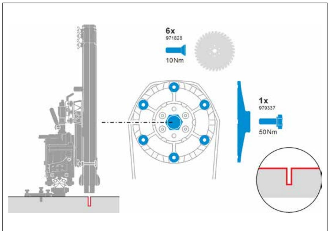
Saw blade mounting for normal cutting
