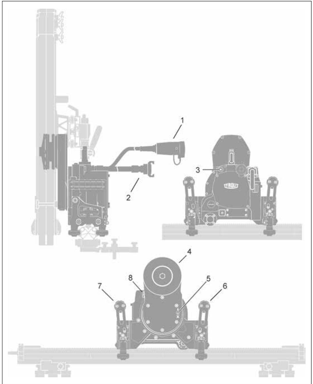
Controls for wall saw head
