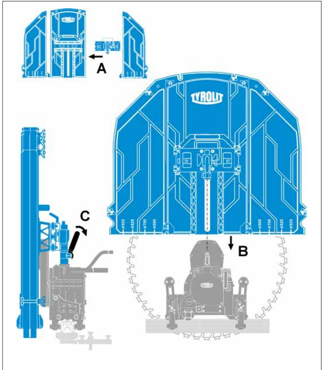
Fitting / removing the blade guard
