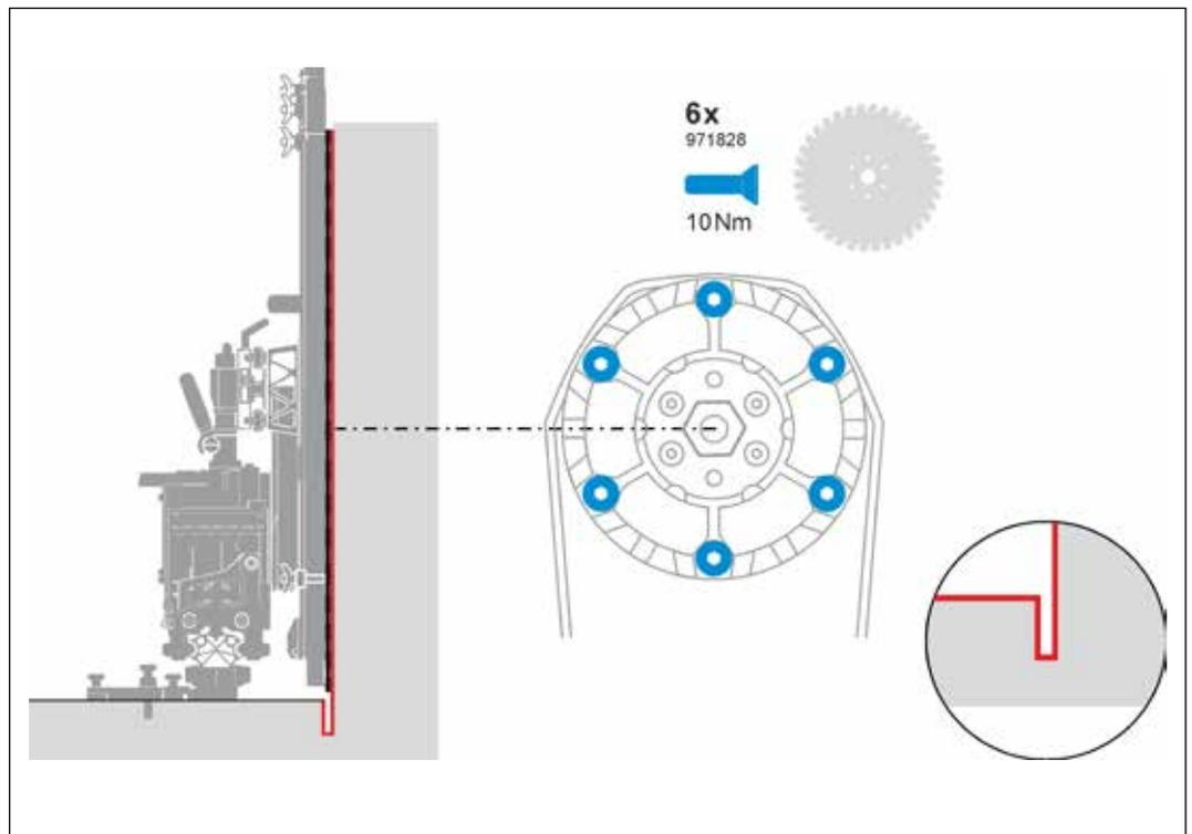
Saw blade mounting for flush cutting
