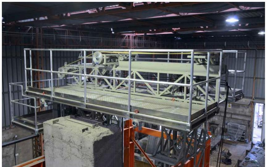
Large, stationary wire saws for the nuclear industry, developed by Studio Corvi.
