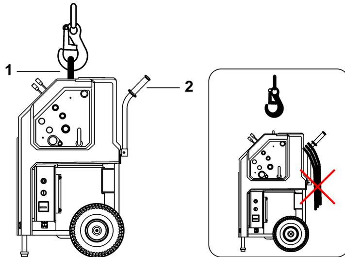
Fig. 8-1 Crane suspension shackle and transport handles
