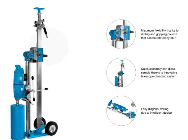
Thanks to its intelligent design with drilling and gripping column that can be rotated by 360°, the DRU350 enables the drilling of holes in walls, ceilings and floors. The drill rig can be mounted in a time saving and material protecting manner via an innovative telescope clamping system. Various settings options, an extended drilling column and a variety of drill accessories ensure universal use.
