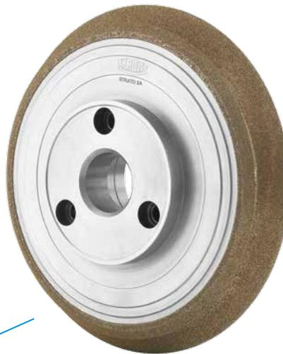
+ **Maximum lifetimes:** A galvanic bond matrix with exceptionally high bond strength keeps the application-specific grain in the bond, even during demanding machining processes. Owing to the special manufacturing process, superabrasives are distributed evenly across the profile and ensure maximum profile retention.
