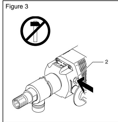
Switch the drill's soft impact feature on or off, depending on the material to be drilled (Figure 2 and Figure 3).
