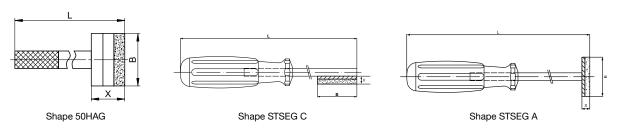
This diamond dresser provides you with a high-quality dressing tool for bench grinding wheels in the precision machining sector. Depending on their design they can be used for peripheral or lateral face machining.
