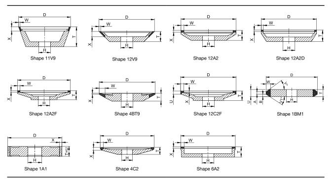
With this tool you can grind all cutting tools for the wood and metal industry and a range of shear blades. These products are disc and cup wheels in the CBN grit size range B181 - B91.
