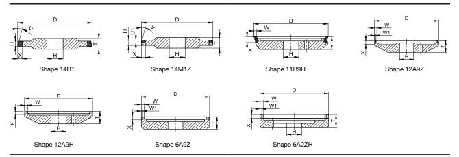
This resin-bonded diamond wheel is available as a cup wheel or peripheral wheel. It is also available as a single or D126/D46 double layer. Double layer wheels achieve an excellent level of cutting quality due to a combination of two grit sizes in a high concentration.
