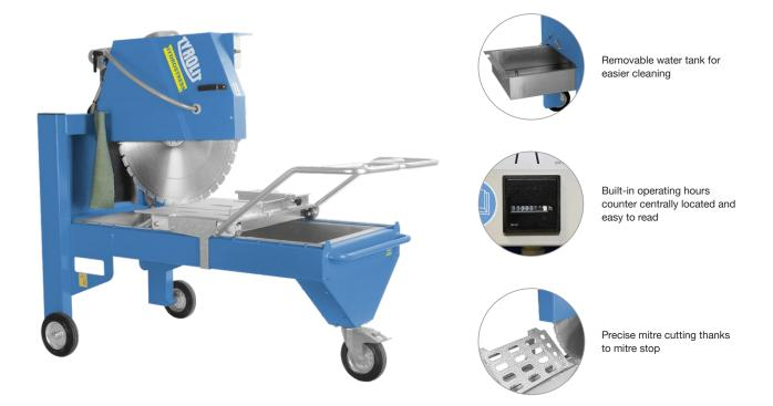
The TME700 convinces through maximum stability and robustness. The precise stainless-steel saw table guide guarantees a clean cut. Construction-site suitable leading pulleys, forklift guides and a crane hook ensure trouble-free transport. The anti-contamination positioning of the water pump reduces servicing requirements to a minimum and ensures permanent tool cooling. The intelligent blade guard construction enables quick and easy blade installation.
