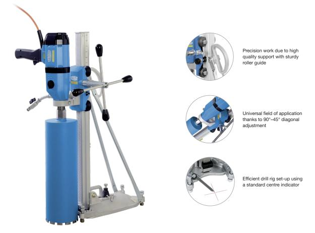
The DRU160 is the lightweight among drill rigs up to Ø 160 mm. The standardised clamping collar system enables quick mounting of common drill motors. In addition, a centre indicator, angle indicator and spirit level enhance user-friendliness and help save valuable time during drill rig set-up. The anchor or vacuum attachment facility also increase flexibility.
