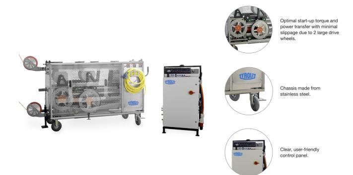
25 m wire storage and a doublemotor high-frequency drive with 37 kW make child's play of decommissioning even large structures likes bridges, chimneys and foundations. The continuously variable wire speed from 0-25 m/s and the precisely adjustable tensile force thanks to pneumatic wire tension help provide optimal cutting performance.
