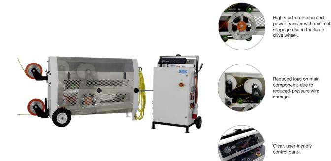
The wire saw has 15 m of wire storage and a powerful 18 kW high-performance drive for tough jobs in high-performance sectors such as controlled dismantling of large buildings. The continuously variable wire speed from 0-25 m/s and the precisely adjustable tensile force – thanks to pneumatic wire tension – help provide maximum cutting performance.
