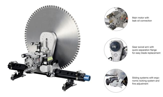
The "work horse" among hydraulic wall saws. Use of the quickseparation flange on the swivel arm provides simple, fast blade replacement and facilitates use in flush cutting applications. With the FZ-4S in conjunction with hydraulic drives with outputs of up to 40 kW, blade diameters of up to maximum 2 200 mm can be used.
