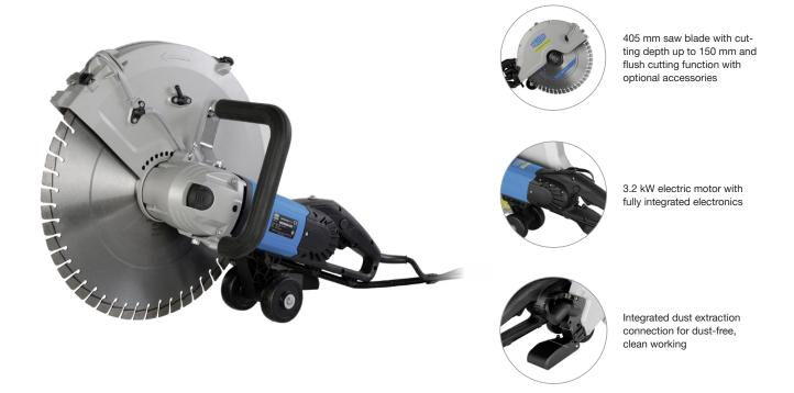
The HBE400 is a 3.2 kW hand-held saw for cutting depths up to 150 mm. In combination with our accessories kit, this hand-held saw is excellently suited to flush cutting. This model can be used for both wet and dry applications and its integrated dust extraction connection enables clean working. The compact design, low weight and detachable guide rollers guarantee ease of handling and machine guidance for the user. The 230 V electric drive enables flexible working indoors and outdoors.
