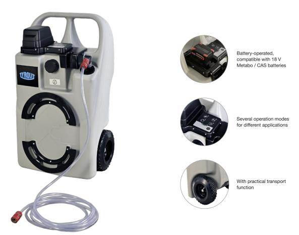
The WTE60 is a large batteryoperated water pressure tank with a 60 litre capacity. With its rechargeable battery and powerful brushless motor, it offers high pressure and delivery performance with a long operating time. It has several operating modes, which are set to core drilling, cutting or cleaning. Its long transparent hose allows easy control of the water flow and can be conveniently stored in the hose holder to save space. Its robust transport wheels make it mobile and flexible to use.
