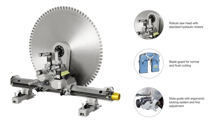
The extremely sturdy and proven design ensures high reliability and cutting accuracy. With the DZ-S2 in conjunction with hydraulic drives with outputs of up to 20 kW, blade diameters of up to maximum 1 200 mm can be used.
