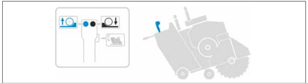
Lifting and lowering the blade
