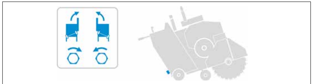
Correcting the tracking (diagram)
