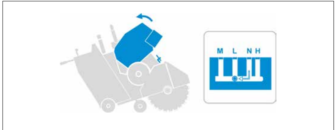
Shifting gears with the 3-speed transmission (diagram)
